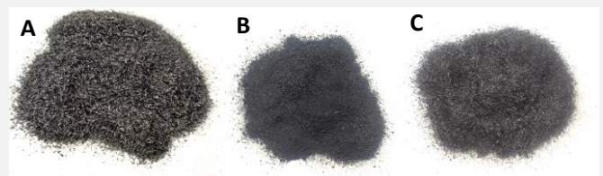
Pinewood biochar pyrolyzed at 500°C (A), 460°C (B), and 700°C (C). Picture credit: Sundar Sapkota
